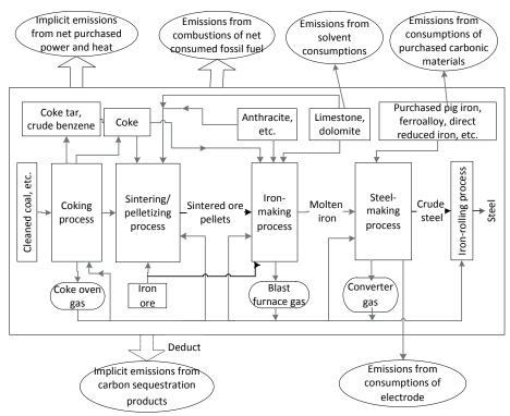
Figure 1 GHG emissions from iron and steel production enterprises and the accounting boundary
